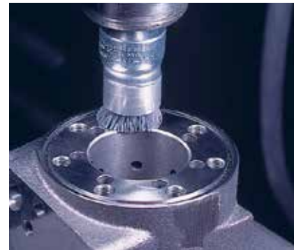
Blending tool marks on a hydraulic component.
