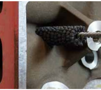
Cleaning burrs out of an automotive head port.
