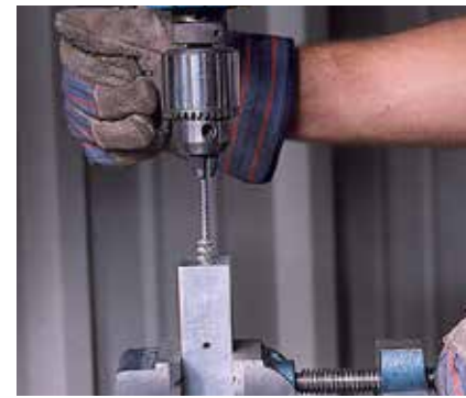
Crosshole deburring an aluminum manifold.
