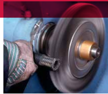
Removing rubber coating from a hydraulic hose.
