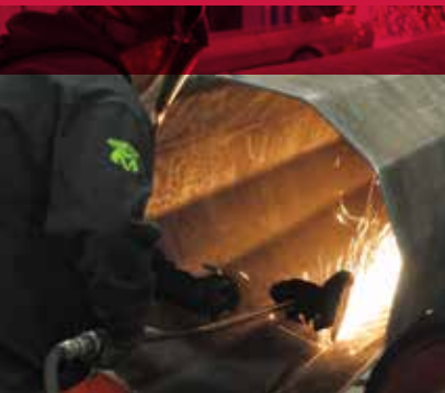
Weld removal with Tiger combo wheel.
