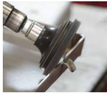
Edge chamfering a fabricated stainless component.
