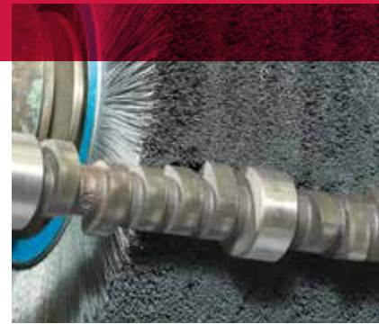
Deburring a camshaft with a Nylox wheel.
