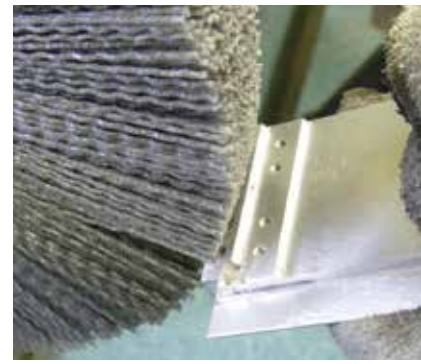
Removing burrs from an aluminum heat sink.
