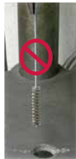
Incorrect Mounting in Chuck
