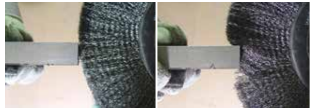
Correct Wire Tips Doing the Work
