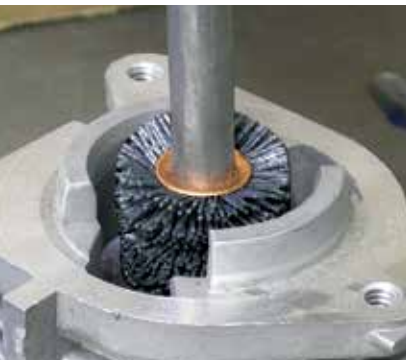
Deburring internal bores of a cylinder head.
