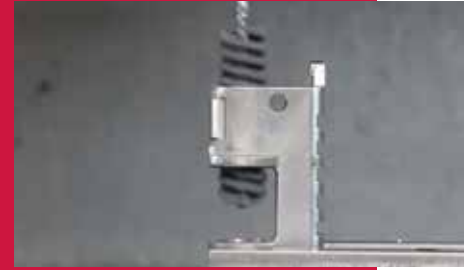
Deburring cross holes in a firearms component.
