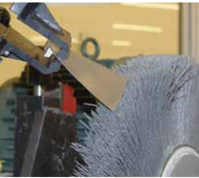
Deburring the tip of a turbine blade.
