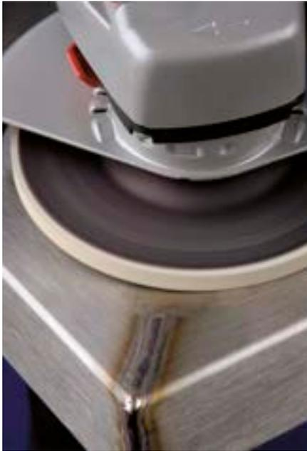
Poliflex® wheels with the textile (TX) bond are manufactured with standard aluminium oxide. The textile fabric inlays make the TX bond a very hard, sturdy bond. Recommended for use on edges.
