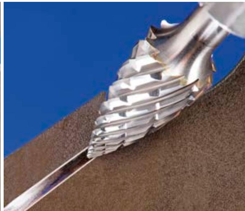
With the INOX cut, PFERD has developed innovative burs for work on stainless steel (INOX). The INOX cut is characterized by an extremely high stock removal rate on all austenitic as well as rust- and acid-resistant steels. It creates significantly less vibration than a comparable cross cut.
