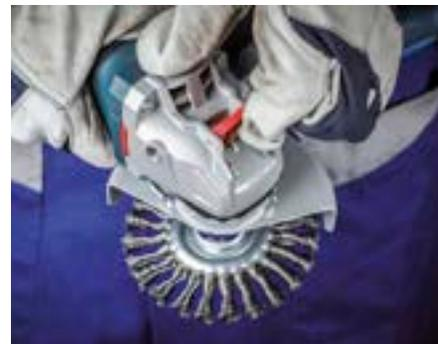
Release the brush by using the lever.
