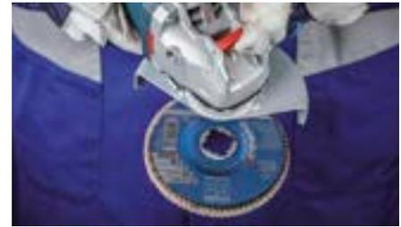
Release the disc by using the lever.
