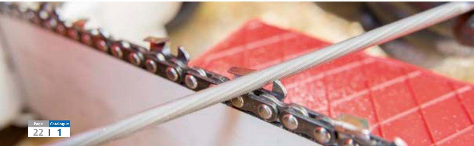
Chain saw sharpeners from PFERD are exceptionally well suited to the manual sharpening of saw chains. Manual sharpening is more economic and much more gentle than machine-based sharpening, and can prolong the service life of the saw chain.
