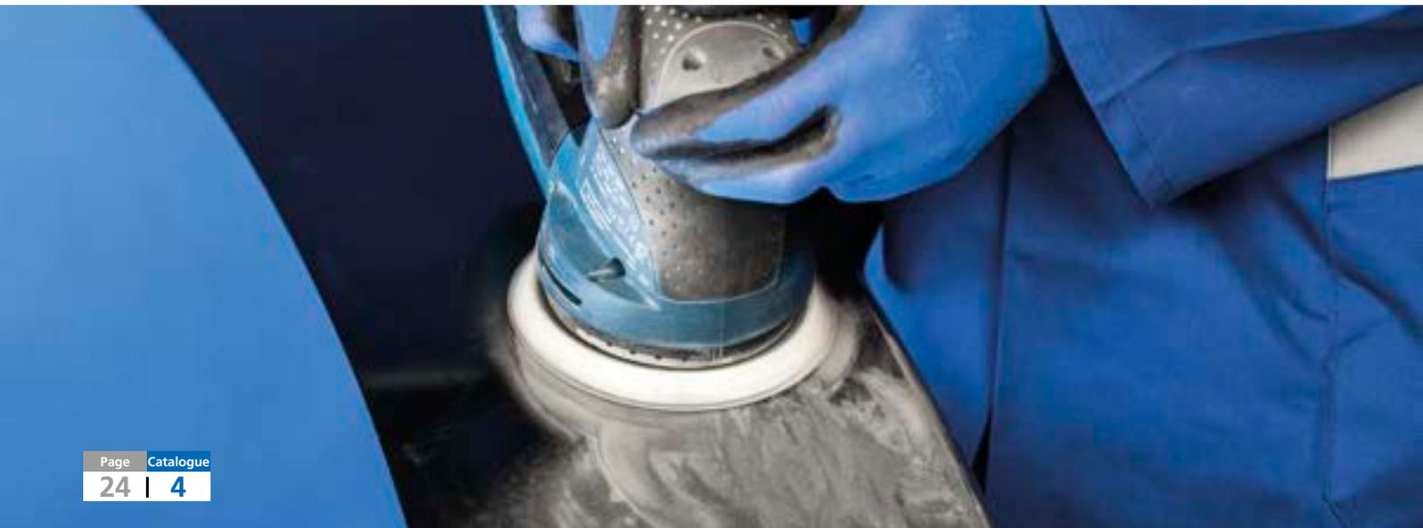
Velcro-backed abrasive discs in the NET type feature a netting fabric, to which the abrasive grain is bonded with a high-performance bond system, which makes it very durable.
