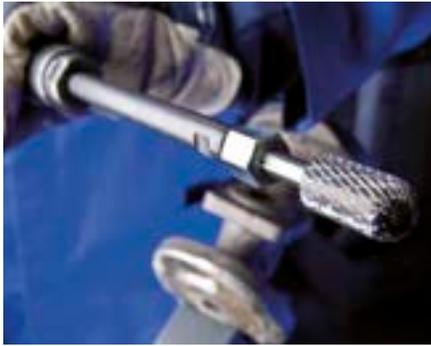
Burs (shank dia. 1/8, 1/4 and 3/8 inch) can be extended with spindle extensions. They allow access to hard-to-reach areas. The drive spindle extension is mounted in the collet of the power tool (air-powered or electric), or in the handpiece of the flexible shaft drive. In some applications, spindle extensions are an economical alternative to customized extended shank burs.
