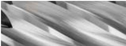
The ALU cut is especially designed for stock removal on aluminum. This cut is characterized by its high stock removal rate.
