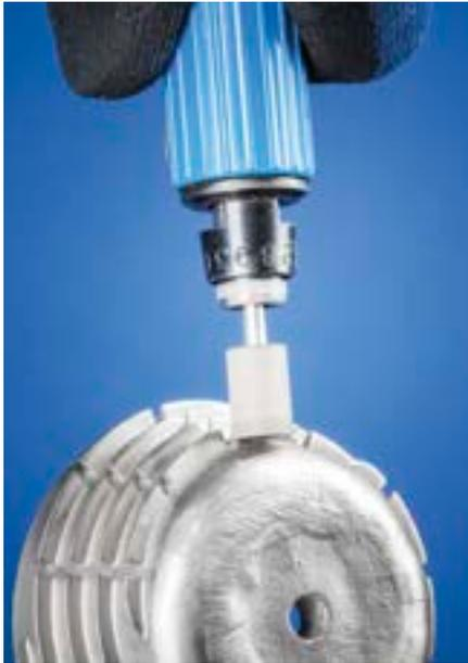
Poliflex® finishing points with the leather bond are manufactured with white aluminum oxide. The leather (LR) bond is a hard, sturdy bond. Ideal for use on surfaces.
