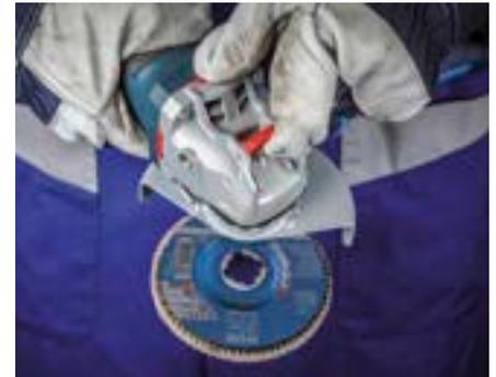
Release the disc by using the lever.
