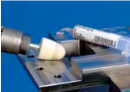
Diamond polishing pastes are used for work on hard materials, such as tungsten carbide and hardened steels. They are used in combination with felt polishing elements. Diamond polishing pastes can be diluted and dissolved with water and alcohol.
