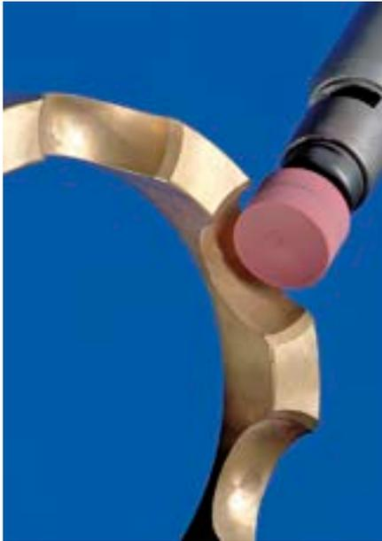
Poliflex® finishing points with the rubber bond are manufactured with pink aluminum oxide. The rubber (GR) bond is an elastomer-based soft bond. Ideal for use on surfaces.
