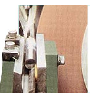
Centerless grinding is a production process that produces extremely close tolerances on metal cylindrical forms or parts. Centerless grinding is used on a wide variety of workpieces. The key components in the process are the grinding wheel, the work rest blade (used to support the work) and the regulating or "feed" wheel (the drive mechanism for the workpiece).
