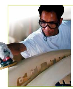
For use on random orbital and rotary sanders. The industry's highest performing film and foam finishing discs are engineered for composite, automotive, and other fine finishing applications. Norton microfinishing film discs produce superior finishes dry without sacrificing cut rate while Norton foam finishing discs are used moist to produce a semi-polished surface to reduce buffing time.
