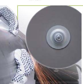
Made from non-woven synthetic fiber mesh, which is impregnated with abrasives and bound with resins, non-woven wheels are designed to create desired surface finish where little or no stock removal is required. The industry's broadest offering is available for light stock removal, deburring, blending, finishing and polishing. Non-woven wheels have an open mesh construction that is waterproof, washable, conformable and non-loading.
