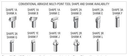
Shapes 3A (F and G Shanks) are used for form, shape, and step truing. Shape 1E is used for angle dressing
