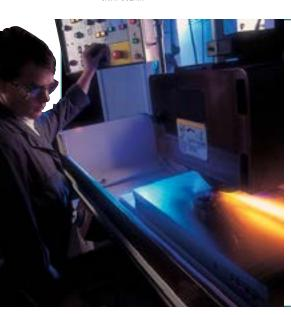
Large surface grinding wheels are generally used to grind flat stock or flat surfaces within a workpiece. These wheels are typically used on horizontal spindle machines. Applications can vary from heavy, rapid stock removal to precision tolerance operations.
