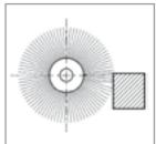
Let the tip of the wire brush do the work – operate the brush with the lightest pressure. If heavy pressure is used, wires will be overstressed, resulting in a wiping action, which, if continued, creates wire fatigue and will shorten brush life. Reversing the rotation periodically sharpens the wire tips for faster cutting action and longer life. Use finest suitable wire size.
