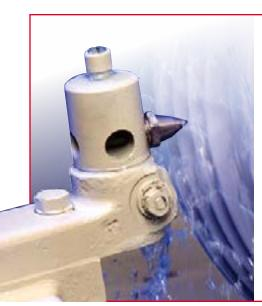
Our Norton Winter offering is the industry's most comprehensive line of stock and made-to-order products to true (restore the wheel's profile) and dress (opening - to remove stock - or closing to finish) the face of the wheel. In addition to these catalog stock stationary tools, Norton Winter manufactures a full line of custom stationary tools, rotary diamond dressers and truing/dressing devices to meet all your specific application needs.
