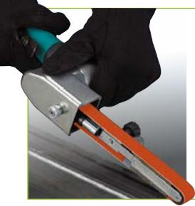
Portable file belt sanders have replaced tedious hand filing and sanding. First introduced in pneumatic, they are now also available in electric. Increasingly, tool manufacturers are introducing additional fixtures for additional applications. The belts listed are popular stock sizes, but additional sizes, specifications, backing materials, and edge scallops are available made-to-order.
