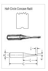
Full-Ball Radius Tools for precision plunge form dressing of concave radii in the center of a grinding wheel are available made to your custom requirements. Ask your Norton representative for details.
