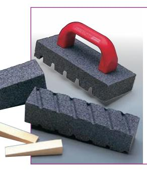
Hard silicon carbide rubbing bricks are used for heavy-duty applications such as rubbing floors, cleaning and scouring castings, rubbing down concrete, and removing mold marks.
