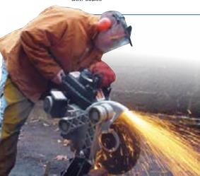
The Norton RailCut line is designed for high-speed fixtured hydraulic or gas-powered rail saws.
