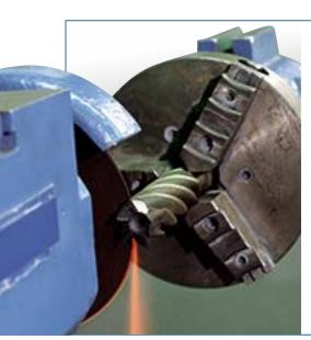
Reinforced and non-reinforced engineered cut-off wheels for cutting all types of tool steel with fixed-based cut-off machines.
