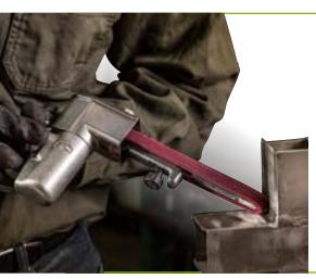
Norton non-woven belts are a combination of strong synthetic mesh and quality abrasive, bonded together by a smear-resistant adhesive. The open construction of non-woven material enables aggressive cutting action and improved surface finish while maintaining its non-loading feature.
