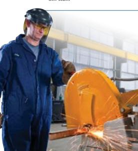
The Norton stationary saw reinforced cut-off wheel line consists of Type 01/41 straight 10" - 24" wheels, designed to fit on fixed-base stationary saws that are free-standing or mounted on a workbench.
