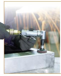
Non-woven quick-change discs are a combination of strong synthetic mesh and quality abrasives, bonded together by a smear-resistant adhesive. The open construction of the non-woven material enables aggressive cutting action and improved surface finish while maintaining its non-loading feature.
