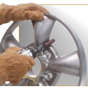
Cartridge rolls are strips of abrasive cloth rolled and glued to form a solid shape that is designed to break down during use and reveal the next layer of abrasive. A valuable abrasive tool for reaching into corners, where larger diameter tools cannot work
