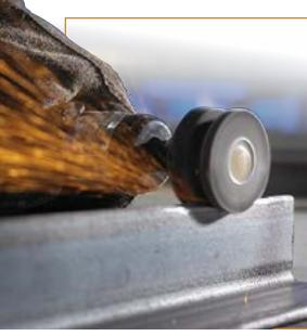
Flap wheels are an ideal choice for a wide variety of blending, deburring and finishing applications common in the metal fabrication, welding and polishing industries. Flap wheels are conformable to intricate shapes and contours. Designed to deliver a consistent finish with a uniform rate of cut, flap wheels wear away, continually exposing fresh abrasives.
