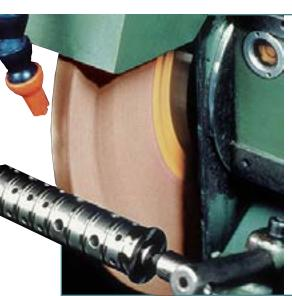
55A-VH blank stock wheels are competitively-priced, monocrystalline grain wheels specifically engineered for numerous carbon steel applications requiring moderate to heavy stock removal rates. They can be altered to your specific needs within two weeks of receipt of your order.
