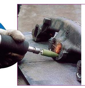
Resin bond, vitrified bond, center lap, and cotton fiber mounted points are available in a wide range of shapes.
