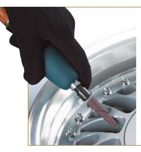
Tapered cone points are strips of abrasive cloth rolled and glued to form a solid shape that is designed to break down during use and reveal the next layer of abrasive. Tapered cone points are similar to cartridge rolls but their shape lends greater accessibility to many difficult-to-reach work areas. They are used for deburring holes and in close tolerance work areas.
