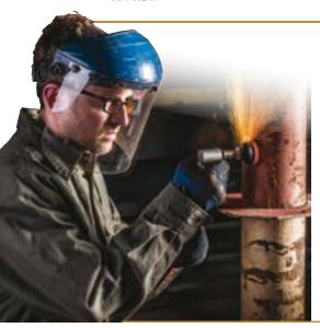
Mini-flap discs are ideal for use in tight spaces. They feature layered flaps which wear away evenly during use exposing new abrasive grain. The lightweight plastic backing helps to absorb vibration. They can help eliminate the conventional 2-step process in grinding edges and removing welds and rust.
