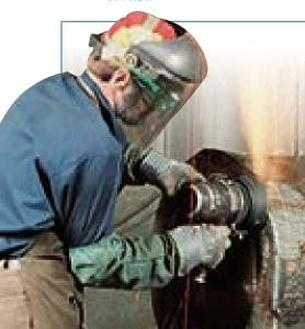
For consistent, quality performance in foundries, welding shops, fabrication facilities, steel mills and shipyards, Norton portable snagging wheels maximize your productivity. Used on horizontal/straight shaft grinders or right angle portable cup grinders.
