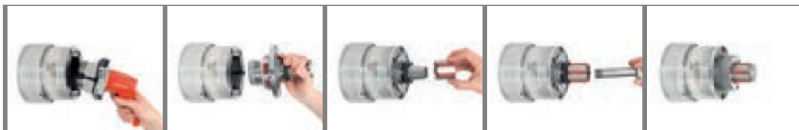
Remove clamping head Insert MANDO Adapt T211 Fit on segmented clamping bushing Screw in draw bolt Clamping device set-up
