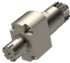
GSC-1110-L Cross Drill/Mill Collet Size: ER16 Output: 1:1 Length 70mm A32
