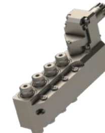
MSE-707 End Drill/Mill Collet Size: ER11 Output: 1:1 External cooling, Requires B-Axis
