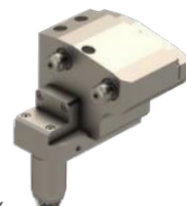
KSE250-KAI-2X End Drill/Mill Collet Size: ER16 Output: 1:2 Internal cooling 30 bar, High speed up to 10,000 RPM *Second Position Is Half Index Drill depth 22mm
