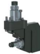
5540-000458 STA-5540-000458 Slitting Saw SR-20R Sub Spindle Tool Size: Ø12.7mm Output: 1:0.55 Adjustable +/- 1mm, Single Ended , Max Tool Ø50mm
