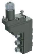
5540-000288 CIT-BSE3209-DE-GSI End Drilling / Milling L32 IX Main Spindle Tool Size: ER11A Output: 1:1 Double Ended
