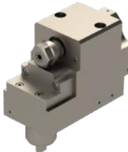
KSE210-IC-V End Drill/Mill Collet Size: ER16 Output: 1:2 Internal cooling, Max 120 bar, Up to 12,000 RPM Drill depth 22mm
