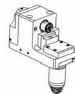
KSE307-1K End Drill/Mill Collet Size: ER11 Output: 1:1 Internal cooling 120 bar, Drill depth 53mm
