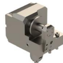
KSS963 Slitting Saw Tool Size: Ø5/8in Output: 8:1 Max Tool Ø: 63mm Max Tool Width: 4mm Requires 2 tool positions
