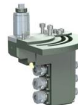
TSU-5540-000258 End Drilling / Milling Main Spindle Collet Size: ER16M, ER11A Output: 1:1 Holds 4 Tools Double-Ended Adjustable 0-90°
