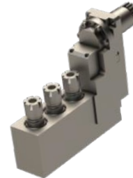
GSA-1510 Angled Drill/Mill Collet Size: ER16 Output: 1:1 Adjustable 0-30°, Requires 2 tool positions A32 L32
