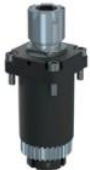
5540-000113 STA-GSC110-GSI Cross Drilling / Milling SR-20JN Sub Spindle Tool Size: ER16 Output: 1:1 Single Ended
