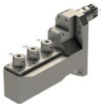
GSE-3607-3M End Drill/Mill Collet Size: ER11 Output: 1:1 Adjustable \pm 30^\circ
