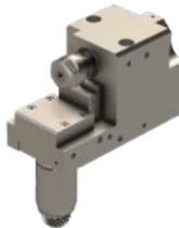
KSE110-DE-32 End Drill/Mill Collet Size: ER16 Output: 1:1 External cooling, Double Ended, Drill depth 25mm front, 17mm back
