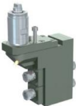
TSU-5540-000218 End Drilling / Milling Main Spindle Collet Size: ER16AM Output: 1:1 Double Ended Holds 4 Tools
