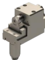
KSE110-KAI-2X End Drill/Mill Collet Size: ER16 Output: 1:2 External cooling 120 bar, High speed up to 10,000 RPM, Drill depth 22mm
