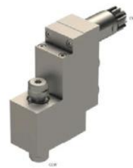
MSE-1007 End Drill/Mill Collet Size: ER11 Output: 1:1 Requires 3 Positions
