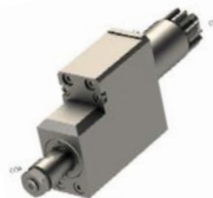
GSS610 Slitting Saw Saw ID: 10mm Output: 1:1 Max Tool \varnothing 40mm Max Width 4.5mm
