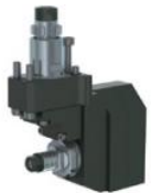
5540-000157 STA-BWSS-5MM Slitting Saw SR-20RIV Sub Spindle Tool Size: Ø5mm Output: 1:0.55 Single Ended, Adjustable +/- 1mm, Max Tool Ø50mm
