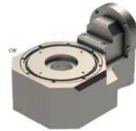
GSW-250 Thread Whirling Ring: Utilis Output: 3:2 3,9, or 12 insert cutter, Adjustable 0 - 25° 6mm Flight Circle Fits manual B-Axis
