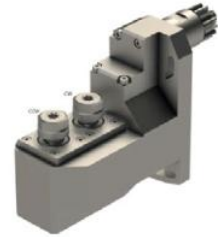
GSE-3607-2M End Drill/Mill Collet Size: ER11 Output: 1:1 Adjustable \pm 30^\circ
