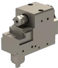
KSE110-IC-V End Drill/Mill Collet Size: ER16 Output: 1:1 Internal cooling, Drill depth 23mm
