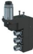
5540-000129 STA-R623131-DE-3E16-11 End Drilling / Milling SR-32JII-A Main Spindle Tool Size: ER16M, ER11M Output: 1:1 Double Ended
