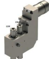
B026-RSE-210-IK Axial Drilling / Milling Collet Size: ER16 Output: 1:1 Double-Ended Internal Coolant-Thru Machine: B026/32/38
