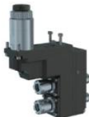
5540-000128 STA-R093-DE2E1611 End Drilling / Milling SR-20JN Tool Size: ER11, ER16 Output: 1:1 Double Ended, ER16 front fac- ing, ER11 back facing
