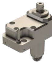
KSC-DEC-10X3 Cross Drill/Mill Collet Size: ER11 Output: 1:3 External cooling, High speed up to 15,000 RPM 10mm Offset
