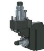
5540-000460 STA-5540-000460 Slitting Saw SR-20RIV Sub Spindle Tool Size: Ø6mm Output: 1:0.55 Single Ended, Adjustable +/- 1mm, Max Tool Ø50mm
