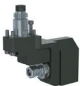
5540-000158 STA-BW-GSC-E11 Cross Drilling / Milling SR-20R Sub Spindle Tool Size: ER11A Output: 1:0.55 Adjustable +/- 1mm, Single Ended
