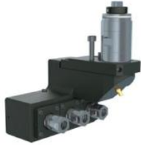
TSU-5540-000240 End Drilling / Milling Main Spindle Collet Size: ER16AM Output: 1:1 Holds 3 Tools
