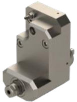
KSC-DEC-L-10x3-V Cross Drill/Mill Collet Size: ER11 Output: 1:3 External cooling, High speed up to 15,000 RPM, 6mm extended
