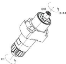
GSC-1110-4X Cross Drill/Mill Collet Size: ER08 Output: 1:3.8 High Speed Spindle A 3 20VII
