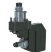
5540-000463 STA-5540-000463 Slitting Saw SR-20RIV Sub Spindle Tool Size: Ø12.7mm Output: 1:0.55 Single Ended, Adjustable +/- 1mm, Max Tool Ø50mm
