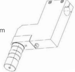
852-354-OF-010 Tool Holder Tool Size: Ø25mm High Speed Spindle Holder
