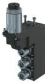
5540-000122 STA-R124-3E16 End Drilling / Milling SB-12 Tool Size: ER16 Output: 1:1 Single Ended, 10mm Flange Thickness
