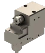
KSE210-V End Drill/Mill Collet Size: ER16 Output: 1:2 External cooling, Drill depth 22mm
