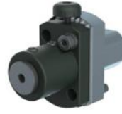
5540-000201 STA-BW-5MM-ADJ Round Shank Tool Holder SR-20R Sub Spindle Tool Size: 5MM Bore Adjustable +/- 1mm Y
