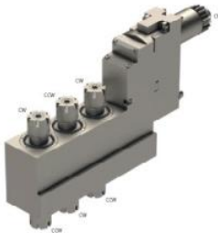
BSA-2010 Angled Drill/Mill Collet Size: ER16 Output: 1:1 Adjustable 0-21° Interferes with adjacent tooling position when used at angle A32 L32
