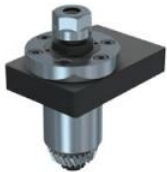
5540-000172 STA-SV20C-E16 Cross Drilling / Milling SV-32JII Turret Tool Size: ER16A Output: 1:1 Single Ended
