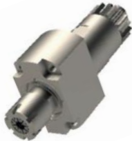
BSC-210 Cross Drill/Mill Collet Size: ER16 Output: 1:1 A32 L32
