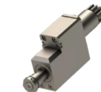
GSS507-08 Slitting Saw Arbor Size: Ø8mm Output: 1:1 Max Tool Ø 50mm Tool Thickness 3mm
