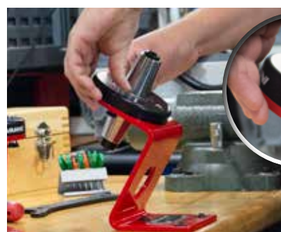
Step 2: Lock-in System + Place thumbs on both buttons. Push down to securely and accurately lock-in tool.
