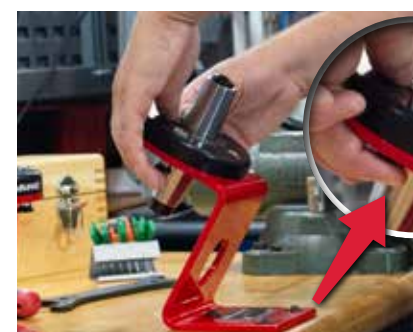
Step 3: Unlock Tool + Place fingers on each securely locked button. Push both buttons upward to quickly and easily unfasten tool.
