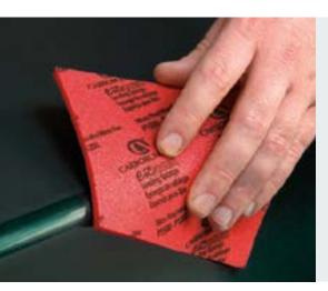
The finishing action of sponges generates a finer finish than conventional coated abrasive products. The coarser grit is the finish achieved when sanding dry and the finer grit is finish achieved when sanding wet.
