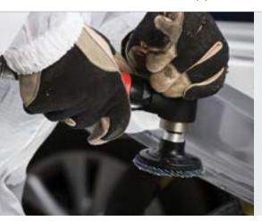
Carbo Premier Red Mini Flap Discs eliminate the conventional 2-step process in grinding, removal, and blending. The abrasive technology used in the Carbo mini-flap discs, combined with the layered flap design, wear away evenly producing a high quality and consistent finish.
