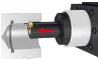
2 Cutter drives into workpiece
