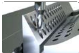
Inclined holes with angle up to 60° on flat surfaces.
