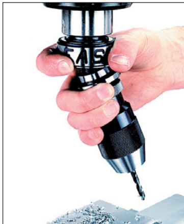
3. Removing drill chuck holder with one hand.
