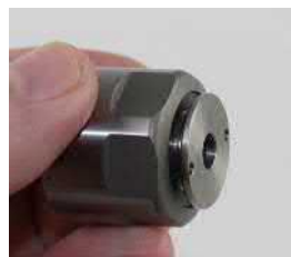
Thread Coolant Cap into ER nut, snug with wrench after the collet has been assembled.
