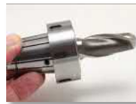
Fully insert cutter into the collet
