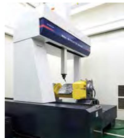
5AX Tilting Rotary Table on 3 Dimensional Measuring Machine
