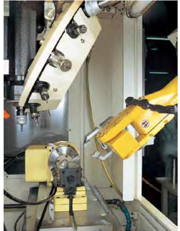
Extremely flexible, and can take many kinds of work pieces. Jig Holder is firmly held in the center hole of CNC Rotary Table as Century Type Holder System. (Simultaneous taper and flange contact) Jig Block can take various work fixtures designed according to each work piece. Plural number of work pieces can be held. Jig Holder with ID is available (optional), and automatic selection of Jig Holder in magazine is possible.
