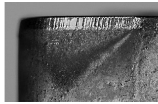
Wear on clearance face
